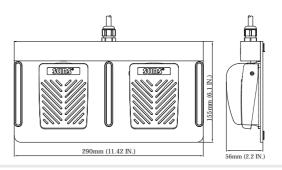
FS-81-SP-(Twin)-2-20/4S (20AWGx4, shielded, 2 meters, 1NO per pedal, cable diameter 7.0mm) FS-81-SP-(Twin)-2-22/5S (22AWGx5, shielded, 2 meters, 1NO per pedal, cable diameter 5.6mm)
