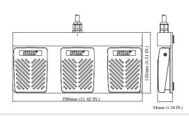
FS-81-SP-(4-Pedal)-2-22/5S (22AWGx5, shielded, 2 meters, 1NO per pedal, cable diameter 5.6mm)
